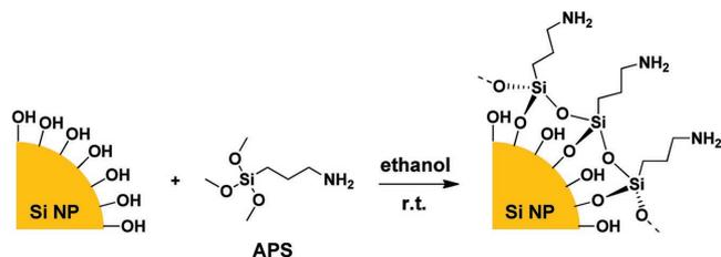
**Scheme 1.** Synthetic route for amine functionalized Si particles. APS was first hydrolyzed to produce silanol (Si–OH) groups, and then silanol groups condense with the hydroxyl groups on Si particles to form covalent Si–O–Si bonds by releasing H<sub>2</sub>O molecules.
