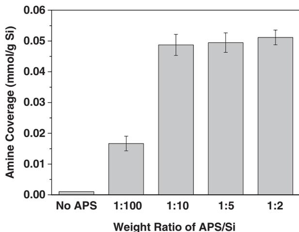
**Figure 1.** Effect of increasing the APS/Si weight ratio in the functionalization bath on the amine coverage of Si–NH<sub>2</sub> nanoparticles.
