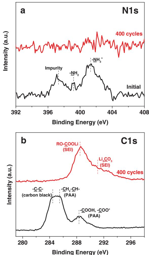
**Figure 5.** XPS spectra of  $\text{Si-NH}_2/\text{PAA}$  anode surface before (black curves) and after 400 cycles (red curves). a)  $\text{N1s}$ , b)  $\text{C1s}$ . The anode was cycled at a current density of  $2.1 \text{ A g}^{-1}$  between 0.01 and 1.0 V versus  $\text{Li/Li}^+$ .
