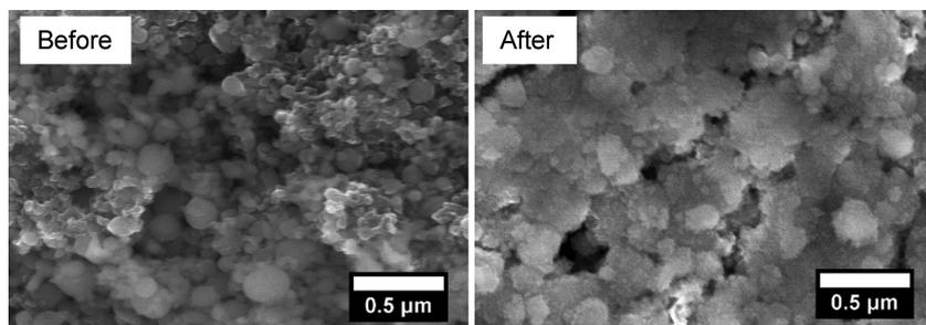
**Figure 4.** Cross-sectional SEM images of  $\text{Si-NH}_2/\text{PAA}$  composite anode before and after cycling. The anode was cycled at a current density of  $2.1 \text{ A g}^{-1}$  between 0.01 and 1.0 V versus  $\text{Li/Li}^+$  for 400 cycles.
