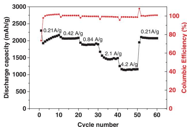
**Figure 7.** Discharge capacity and Coulombic efficiency of Si-NH<sub>2</sub>/PAA composite anode at various current densities cycled between 0.01 and 1.0 V versus Li/Li<sup>+</sup>. The capacity was normalized by the weight of Si particles. Si nanoparticles in this study have amine coverage of  $0.050 \text{ mmol g}^{-1}$  Si.
