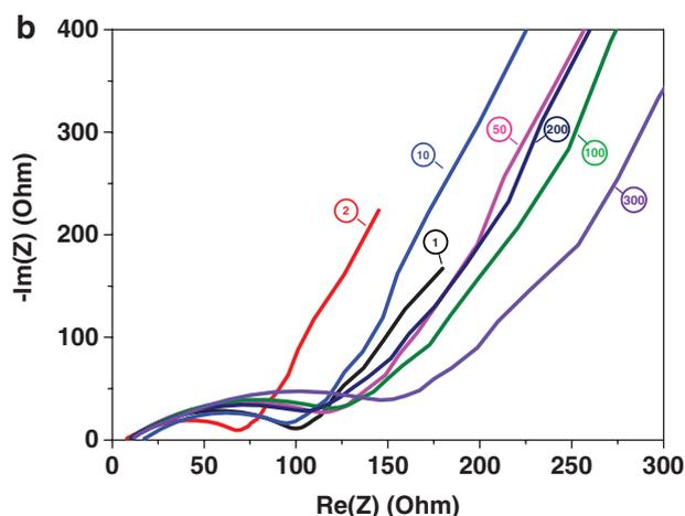
**Figure 8.** Impedance testing results for a) Si-NH<sub>2</sub>/PAA and b) Si/PAA composite anode. The anodes were cycled at a current density of  $2.1 \text{ A g}^{-1}$  between 0.01 and 1.0 V versus Li/Li<sup>+</sup>. The circled number refers to the cycle number of galvanostatic cycling and impedance was measured after completion of the entire discharge/charge cycle. Si nanoparticles in Si-NH<sub>2</sub>/PAA anode have amine coverage of  $0.050 \text{ mmol g}^{-1}$  Si.
