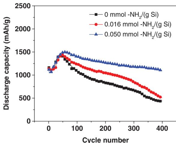
**Figure 6.** Electrochemical cycling performance of Si composite anodes with different amine coverages on Si particles. The anodes were cycled at a current density of  $2.1 \text{ A g}^{-1}$  between 0.01 and 1.0 V versus Li/Li<sup>+</sup>. The anodes were preconditioned with a single formation cycle at a current density of  $0.175 \text{ A g}^{-1}$  (results not shown). The capacity was normalized by the weight of Si particles.
